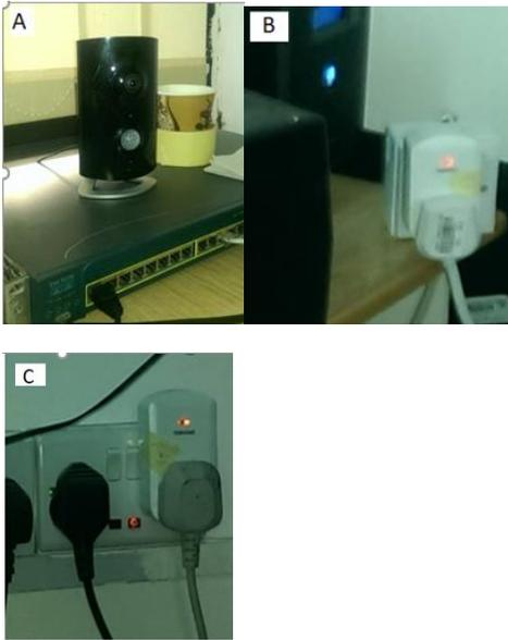
Fig. 2. Picture of the WSAN components (a) Wave presence detector (b, c) Energy Monitor
