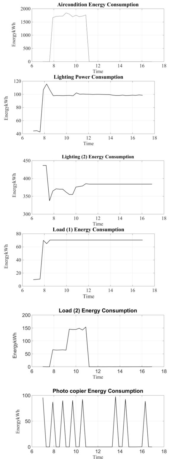
Fig. 3. The energy consumption for different loads in one working day
